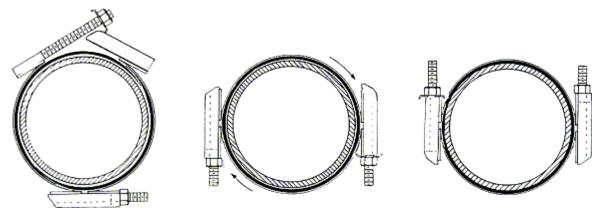
Concord clamps are completely preassembled. The "open finger" design provides easy handling and allows:
