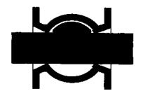
In the full-open position, the plug is rotated out of the main fluid stream as shown. This allows for high capacity flow through the valve.
