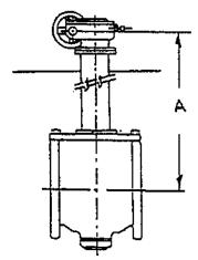
**EXTENDED BONNET ASSEMBLY VALVES FOR** BURIED OR SUBMERGED SERVICE. CAN BE FURNISHED WITH HANDWHEEL/GEAR, CYLINDER OR ELECTRICAL ACTUATOR.
