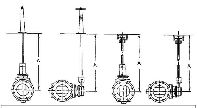
FLOORSTAND INSTALLATION WRENCH OPERATED ACTUATED VALVE VALVE
