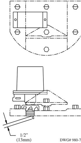
**Typical Pressure Reducer Type Valve Installation**
