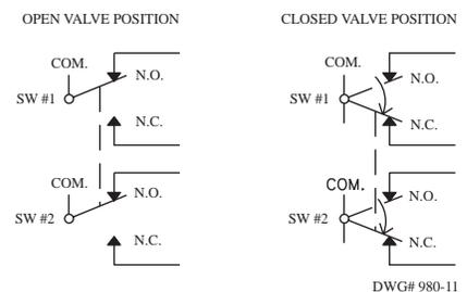
Switches Shown in Valve Open Position
