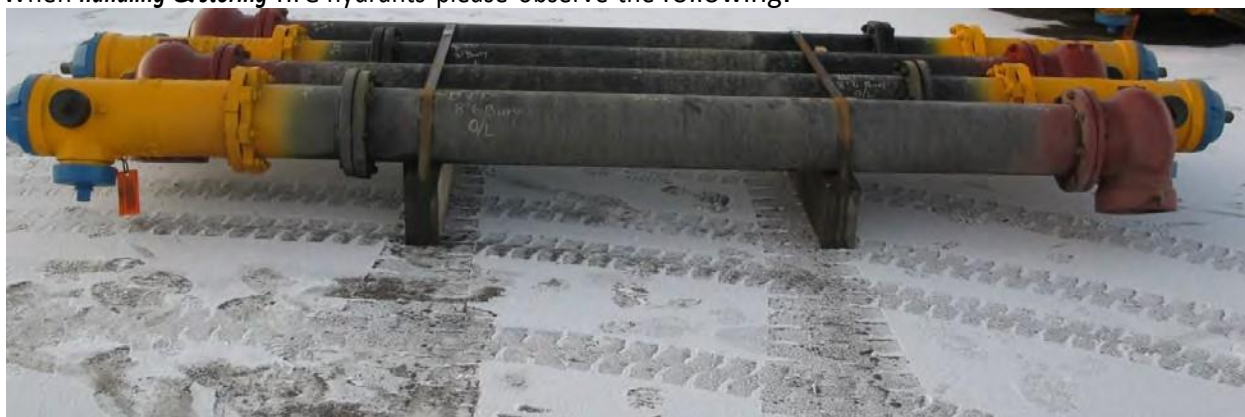
8'6" bury hydrants shown above
